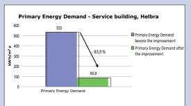
cal measures, including roof and external wall insulation, the replacement of windows and the installation of solar panels for hot water and heating.
